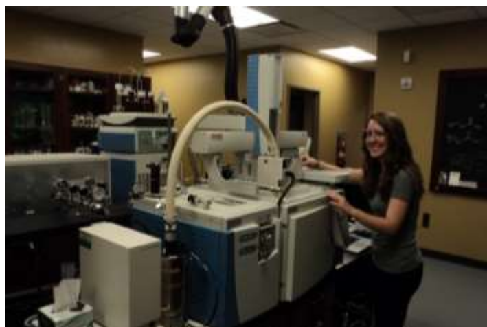
Figure 2. Thermo Trace GC Ultra with ISQ single quadrupole MS being operated by Butler University undergraduate summer research fellow Jericha Mill.
