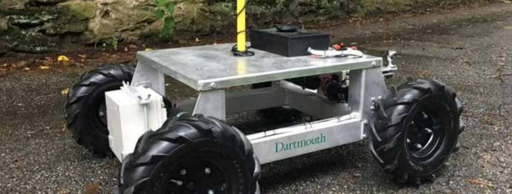
The Archaeorover improves geophysical surveying for archaeological research. —Dartmouth College
