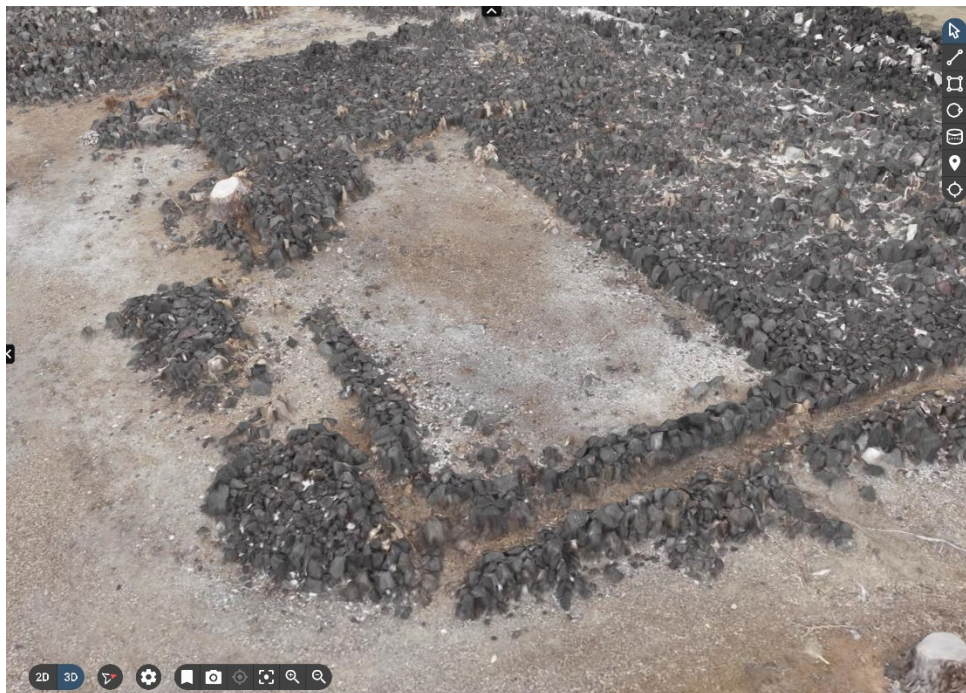
Figure 5-6. A 3D mesh representation of rock walls with a surface texture draped over the fine scale mesh model3D Point Cloud Production.
