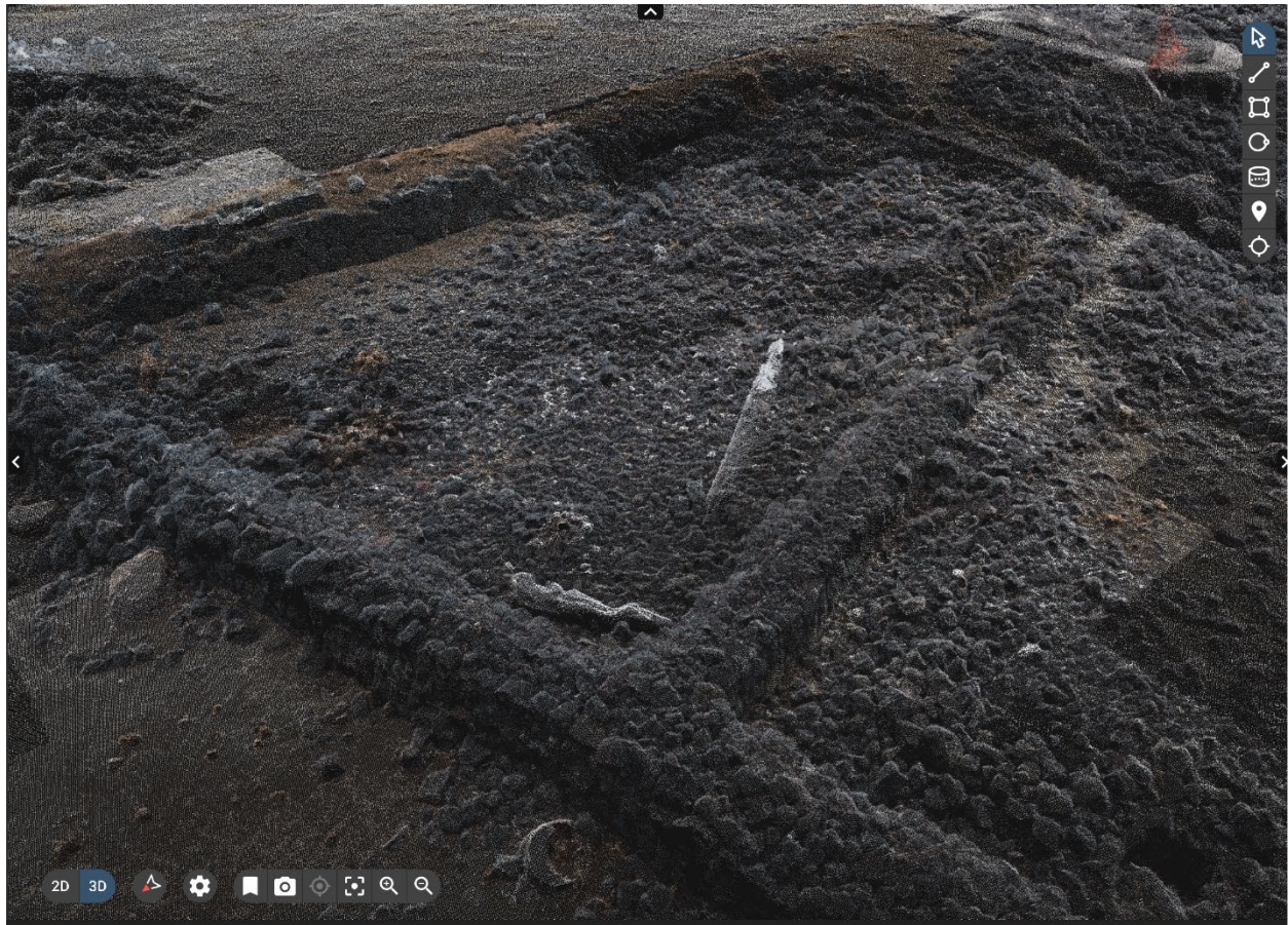
Figure 5-3. Walls rendered as a point cloud using photogrammetry.
