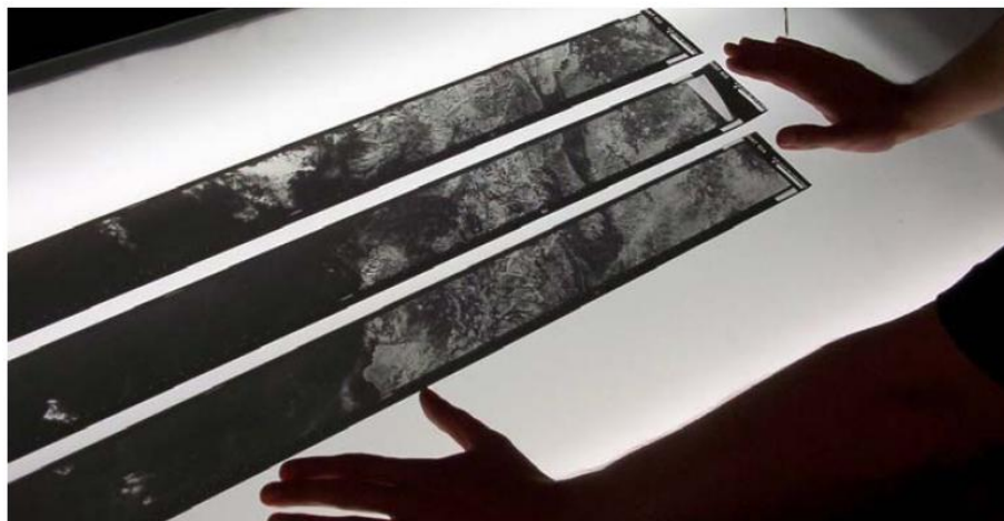
Figure 10: Original CORONA film strips like those pictured above contain extreme spatial distortions caused by the satellites' panoramic camera systems.
