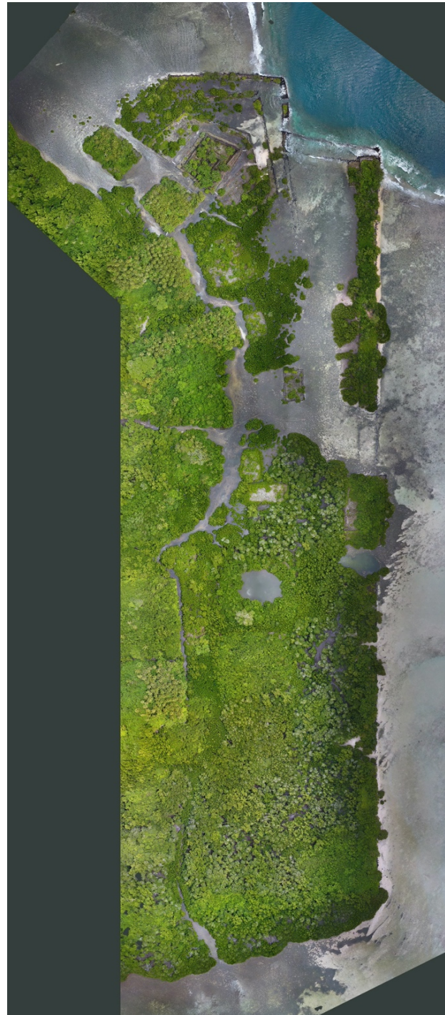
Figure 1 Orthomosaic created from Structure-from-Motion photogrammetry of Nan Madol World Heritage Site in Pohnpei produced by Dr. Andrea Jalandoni and Maria Kottermair from UAS.
